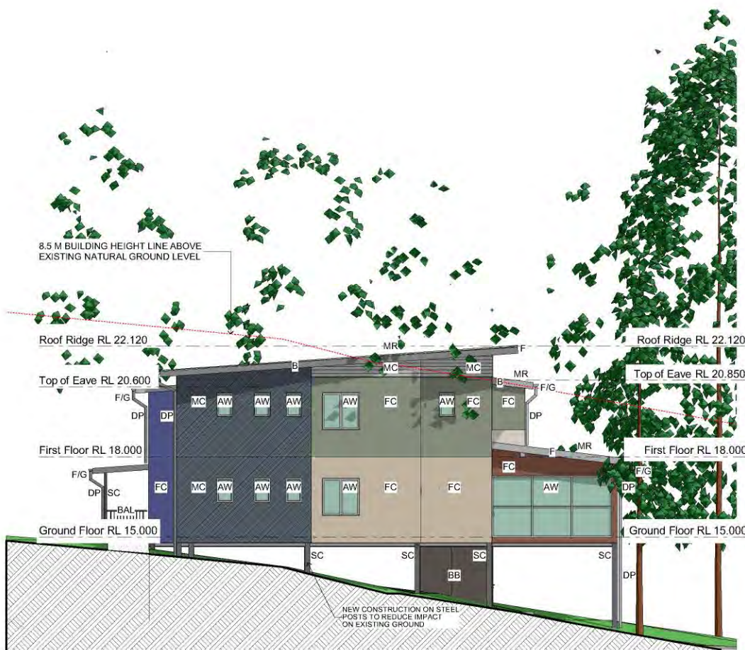
4 Cabin 4 - East Elevation 1:100
