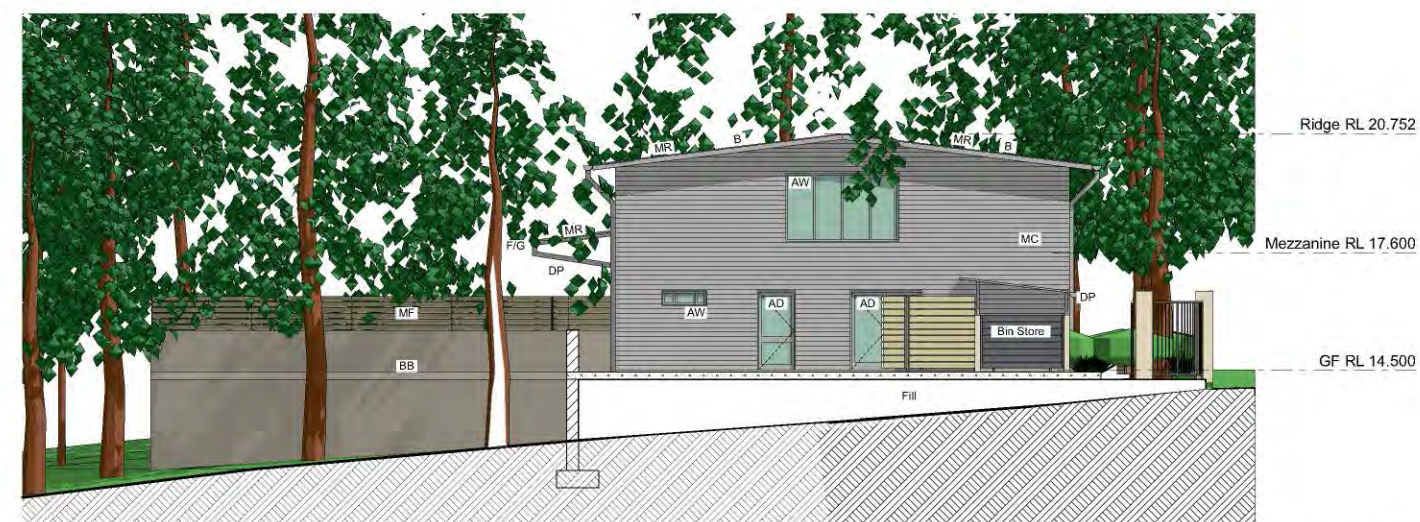
3 Maintenance Shed - South Elevation 1:100
